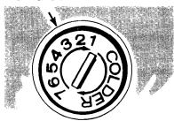
Set cold control – Insert a coin in the slot of the control to turn it. To start, turn cold control to Number 3. This position will maintain zero zone temperatures under normal operating conditions. Turn the cold control to a higher number for colder temperatures or a lower number for less cold temperatures.
